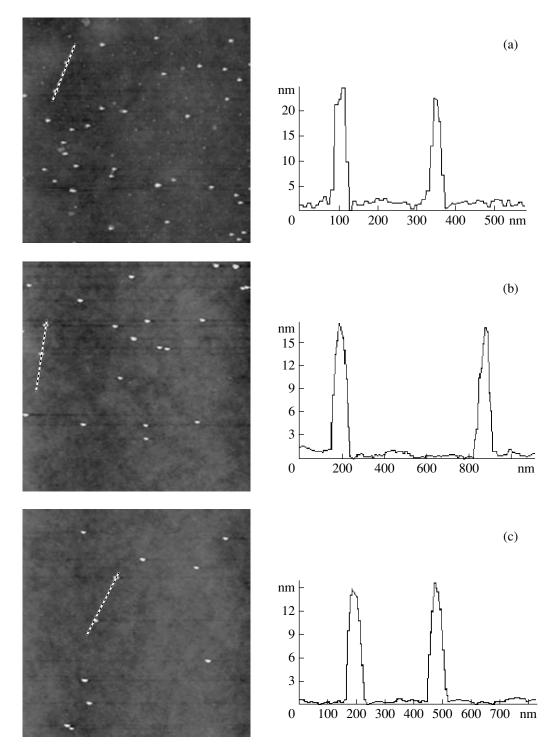
Fig. 7. The AFM images and the corresponding cross sections of the surfaces of PS-234 and its mixtures with PS-5 oligomer covered with adsorbed gold nanoparticles after the sample exposure at room temperature: (a) PS-234, (b) 2 and (c) 5 vol % of PS-5. The scan area is  $2 \times 2 \,\mu m^2$ .
