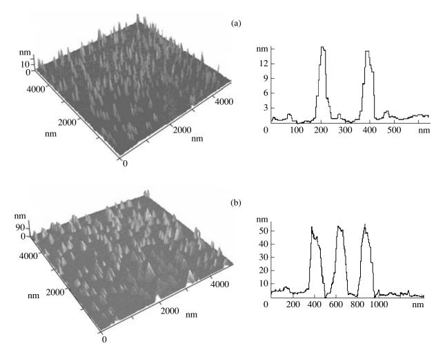
**Fig. 8.** The AFM 3D images of the surfaces of PS-234 surface with adsorbed gold hydrosol particles after (a) the annealing of a system at 60°C for 1 h and (b) consequent exposure in the solution of  $HAuCl_4/NH_2OH$  mixture for 9 min and the corresponding cross section of the surface relief.
