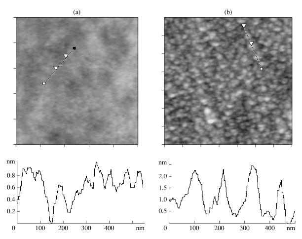
Fig. 4. The AFM images of the surfaces of bare (with no nanoparticles) PVP films after their dipping in (a) water and (b) the solution of HAuCl<sub>4</sub>/NH<sub>2</sub>OH mixture for 9 min and the corresponding cross sections of the surface relief. The scan area is  $2 \times 2 \,\mu m^2$ .
