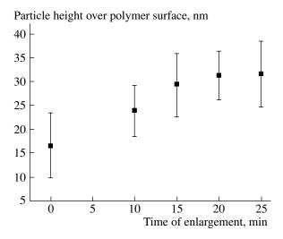
Fig. 6. The kinetics of the enlargement of Au nanoparticles on the PVP surface.
