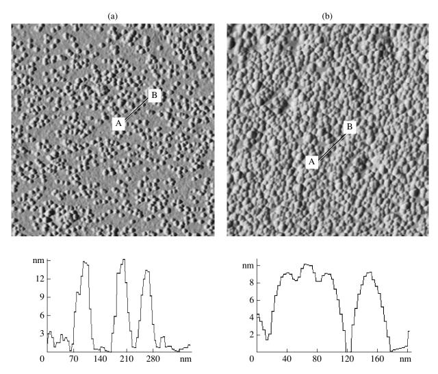
**Fig. 2.** The AFM images of the surface of poly(2-vinylpyridine) after the adsorption of gold hydrosol particles for (a) 10 min and (b) 1 h. Corresponding cross sections of the surface relief are shown below. The scan area is  $2 \times 2 \,\mu\text{m}^2$ .
