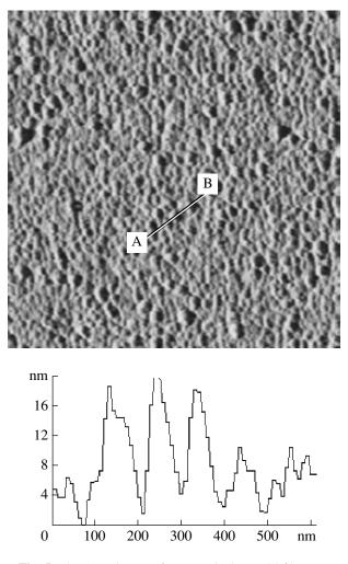
**Fig. 5.** The AFM image of nanoparticulate gold film prepared by the dipping of sample 2 in the solution of HAuCl<sub>4</sub>/NH<sub>2</sub>OH mixture for 9 min and the cross section of surface relief along the AB line. The scan area is  $2 \times 2 \,\mu m^2$ .
