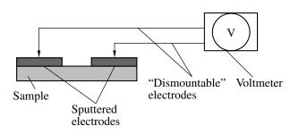
Fig. 1. Block diagram of a device for measuring conductivity of colloidal gold film on the surface of glassy polymer.
