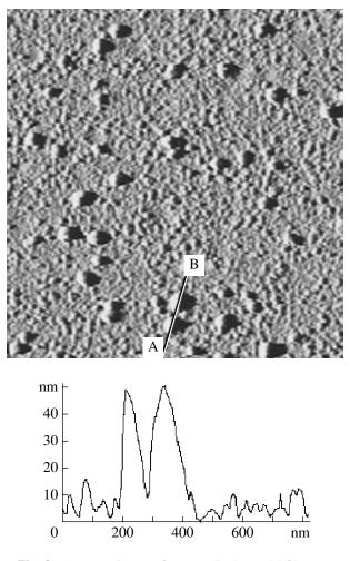
**Fig. 3.** The AFM image of nanoparticulate gold film prepared by the dipping of sample 1 in the solution of HAuCl<sub>4</sub>/NH<sub>2</sub>OH mixture for 9 min and cross section of the surface along the AB line. The scan area is  $2 \times 2 \mu m^2$ .
